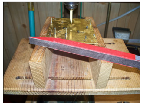
Figure 16. A second alternate approach to restoring a taper—using a sanding stick.
