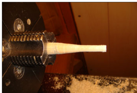
Figure 5. A dowel tapered to do several larger holes. The dowel is cut to be just too big to just slide into the holes—so that the outer edge of the peg is sheared off as it is spun into the holes.
