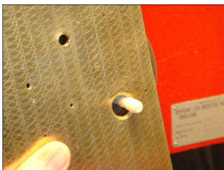
Figure 10. Polishing the inside of a tapered hole.
