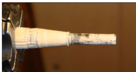
Figure 8. Residual on peg after doing both strike drum carriers.
