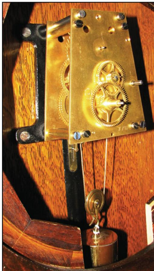
**Figure 2, left.** The movement and pendulum are mounted in the case—no access is available.
