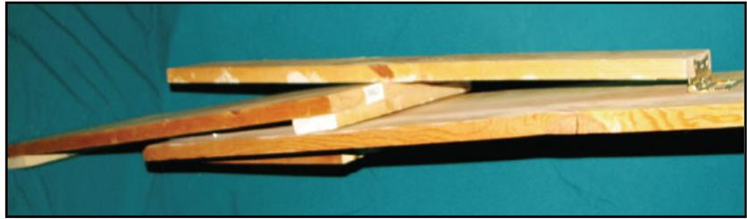
**Figure 4.** Portable test stand collapsed into storage position.
