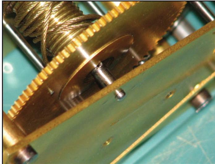
**Figure 5.** The pin through the arbor on the cable winding shaft had metal fatigue, was bent just a little, and allowed too much play.
