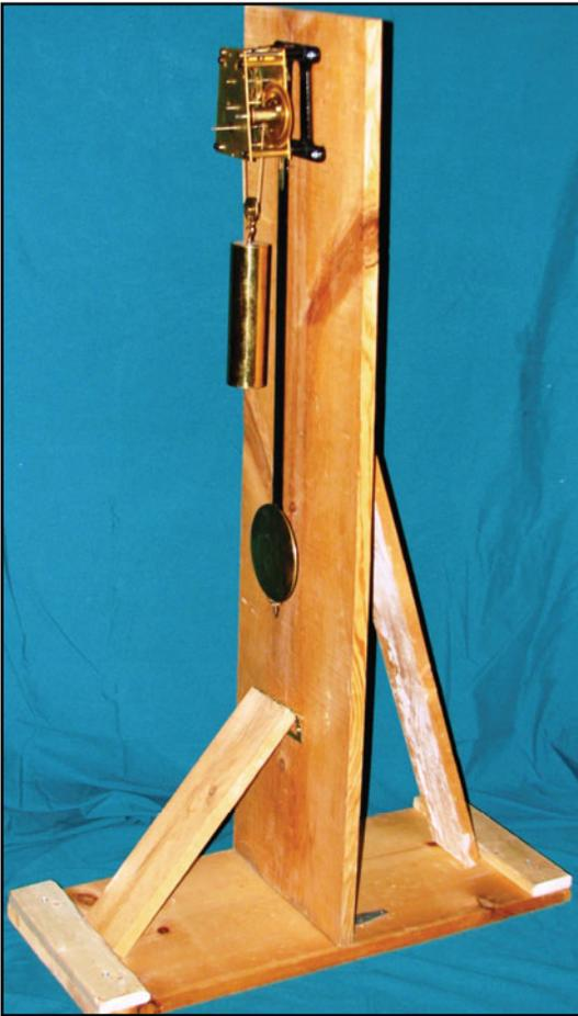
**Figure 3.** The finished test stand with movement and pendulum in place.
