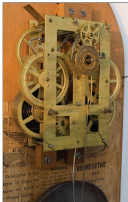
Figure 23. Left front \frac{3}{4} view of movement of Figure 21. The alarm escape wheel has holes to save brass. Note one, not two, slots in count wheel, and two notches in drop slot disc of alarm third wheel. The rims of both time and alarm great wheels are about the same width. See text.
