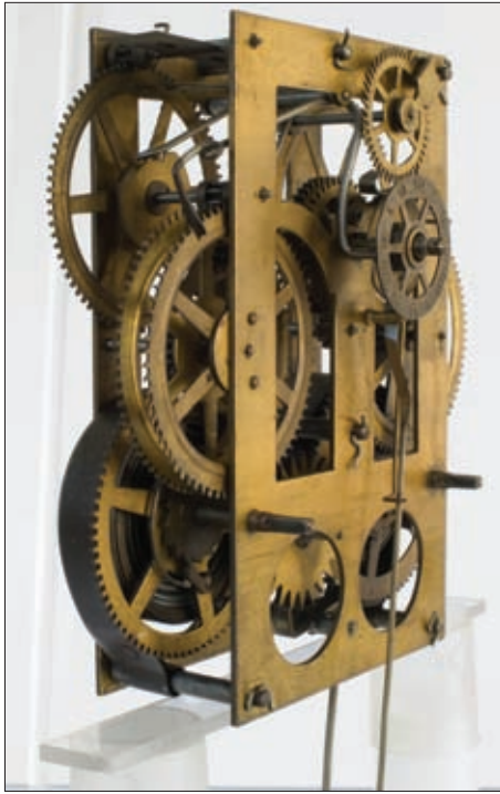
Figure 16. Left front \frac{3}{4} view of movement of Figure 14, showing alarm detent in notch of alarm set wheel. Note two notches in drop slot disc of alarm third wheel. See text.
