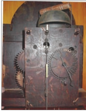
Figure 25C. Back of backplate of movement of clock of Figure 25A, typical for Ireland movements.
