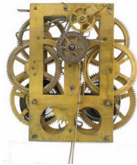
Figure 14. Movement of timepiece of Figure 12. Note two, not one, slots in count wheel. See text.
