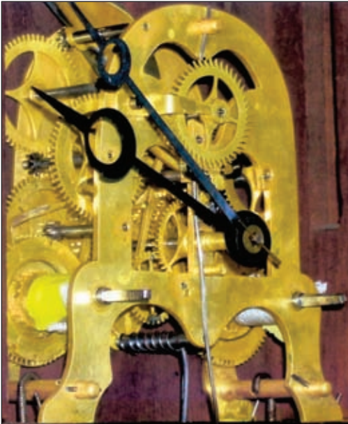
Figure 2. Unidentified 8-day brass time and strike movement found in Clock X. Plates are cast brass. Back plate is solid.
