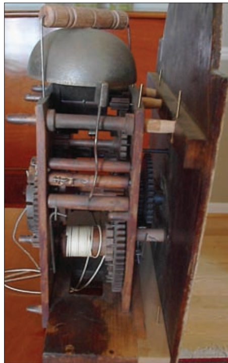
Figure 25E. Left (strike) side view of movement of Figure 25A. The arrangements supporting the function of the hammer arbor are a later development in Ireland movements. See text.
