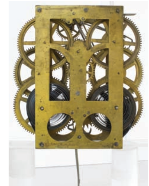
Figure 15. Back of movement of Figure 12. Note rim of alarm great wheel narrower than that of time great wheel. See text.
