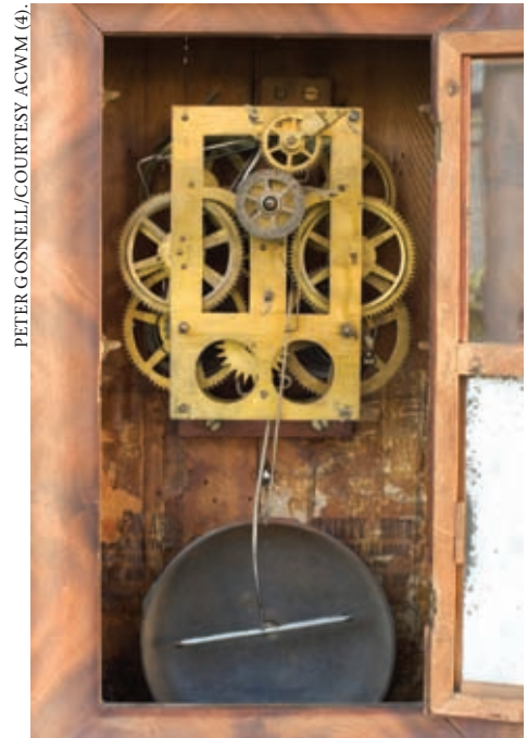
Figure 13. Timepiece of Figure 12, door open and dial removed, showing bell and mostly unreadable label below, and movement above. Best guess as to movement manufacturer could be New Haven Clock Co.
