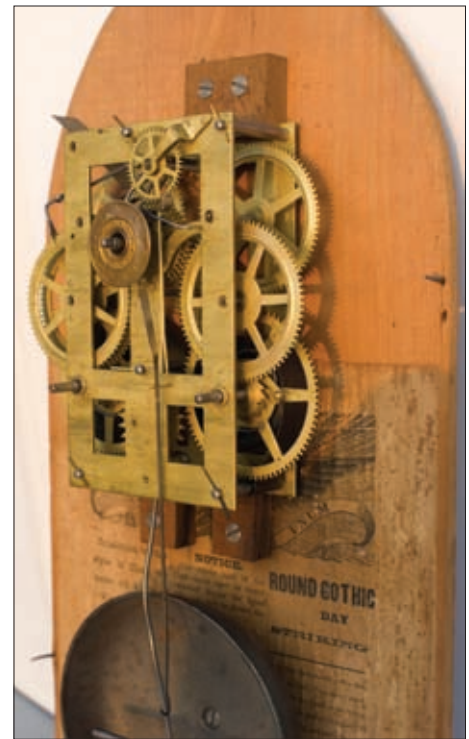
Figure 24. Right front \frac{3}{4} view of movement of Figure 21. Note the new style escape cock (compare to old style Figure 14).
