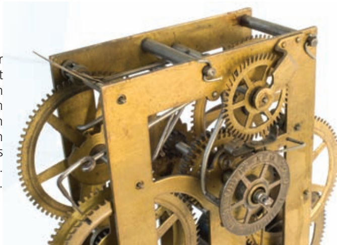
Figure 16. Left front \frac{3}{4} view of movement of Figure 14, showing alarm detent in notch of alarm set wheel. Note two notches in drop slot disc of alarm third wheel. See text.
