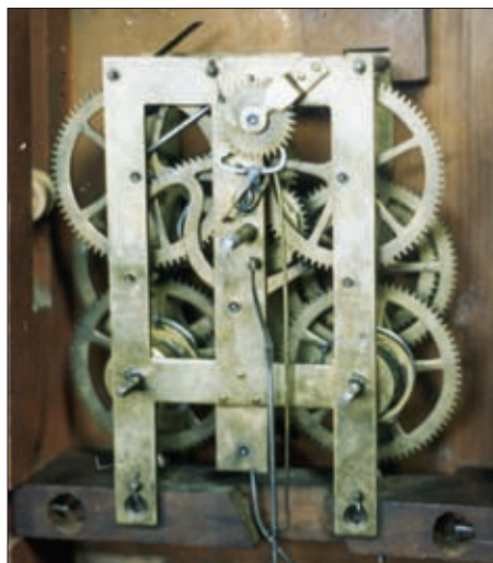
Figure 4, above. Eight-day brass time and rack and snail strike movement found in the Smith clock shown in Figure 3. This is identified as a minor variation of a product of C. & N. Jerome, ca. 1837-1839. At least two Smith or Smith-attributed cases have been found with these similar movements.
