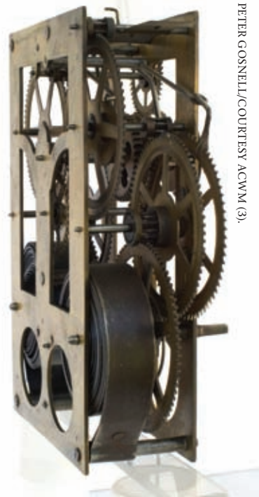
Figure 17. Left back \frac{3}{4} view of movement of Figure 14 showing 12L pinion of alarm second wheel; in contrast, will have 8L pinion on second time wheel. See text.
