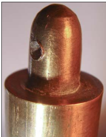
Figure 3. Rough pillar pin hole.
