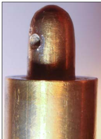
Figure 4. Shard removed from around pin hole.
