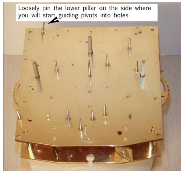
Figure 7. Which pillar to loosely pin first?
