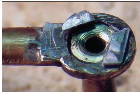
**Figure 4.** Hub fluxed and ready to solder.
