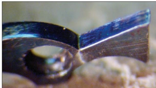
**Figure 13.** Showing solder penetration into crack.
