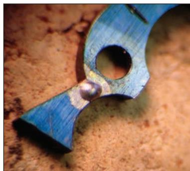
**Figure 12.** Click after heating to melt solder.
