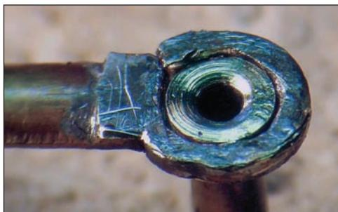
**Figure 2.** Hub ready to be soldered.
