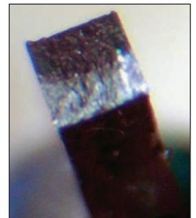
**Figure 9.** Half of the click's broken face is blued—showing that it was broken half way through when heat-blued by the author.
