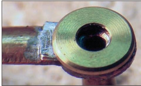
**Figure 6.** Reinforcing washer in place.
