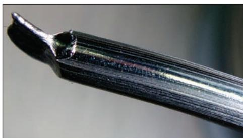
**Figure 3.** Silvabrite 100 solder compressed to make it easier to cut off a very small piece.
