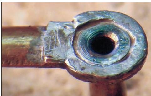
**Figure 5.** Soldered hub.
