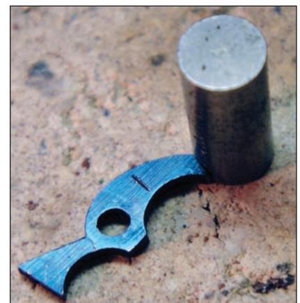
**Figure 10.** Two parts of broken click held in place by a magnet.
