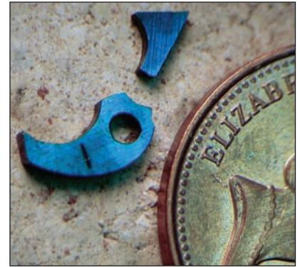
**Figure 8.** Broken winding drum click. British penny shown for scale.
