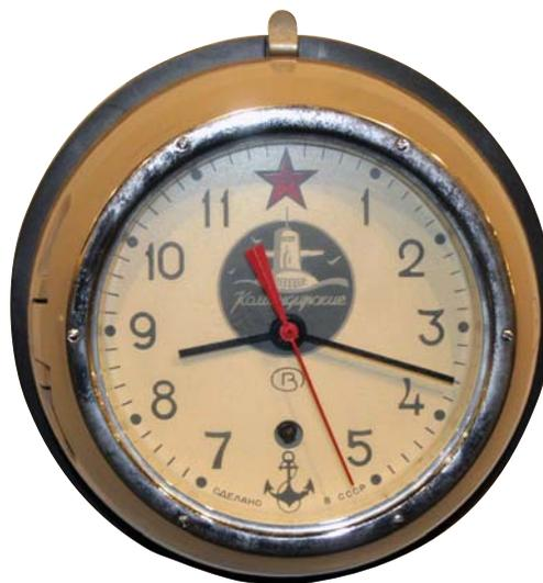
Ship's clock. Russian lettering on lower dial translates "Made in the USSR." Diameter 8.5 in.; depth 3.5 in.
