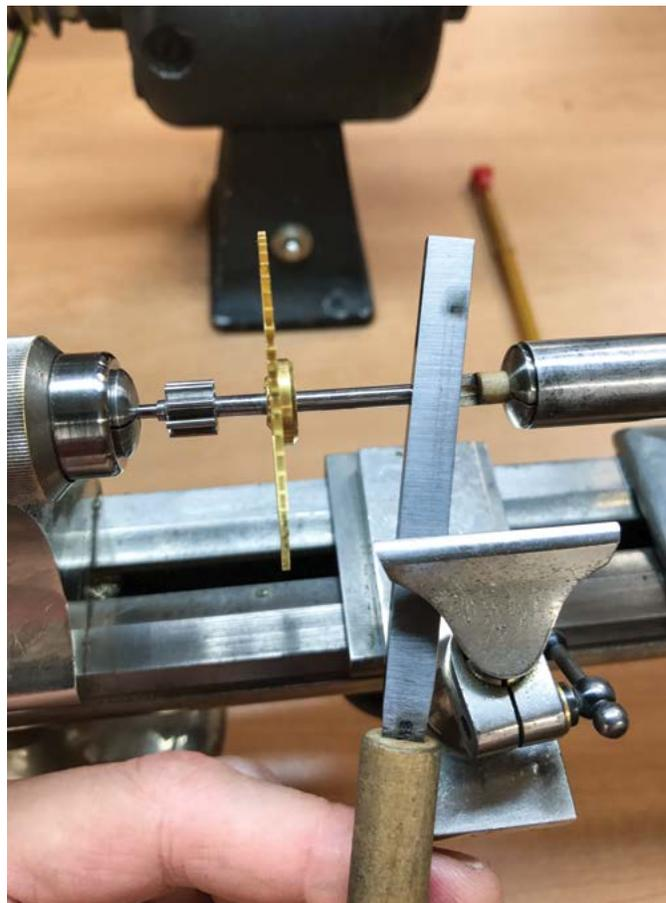
**Figure 2.** Darkening oil indicates that the burnisher is polishing.
