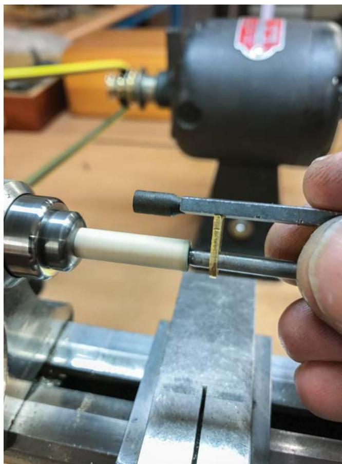
**Figure 10.** Final polishing on inaccessible pivot.
