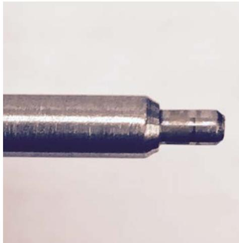
**Figure 4.** Same pivot as in Figure 3 but before dressing and polishing.
