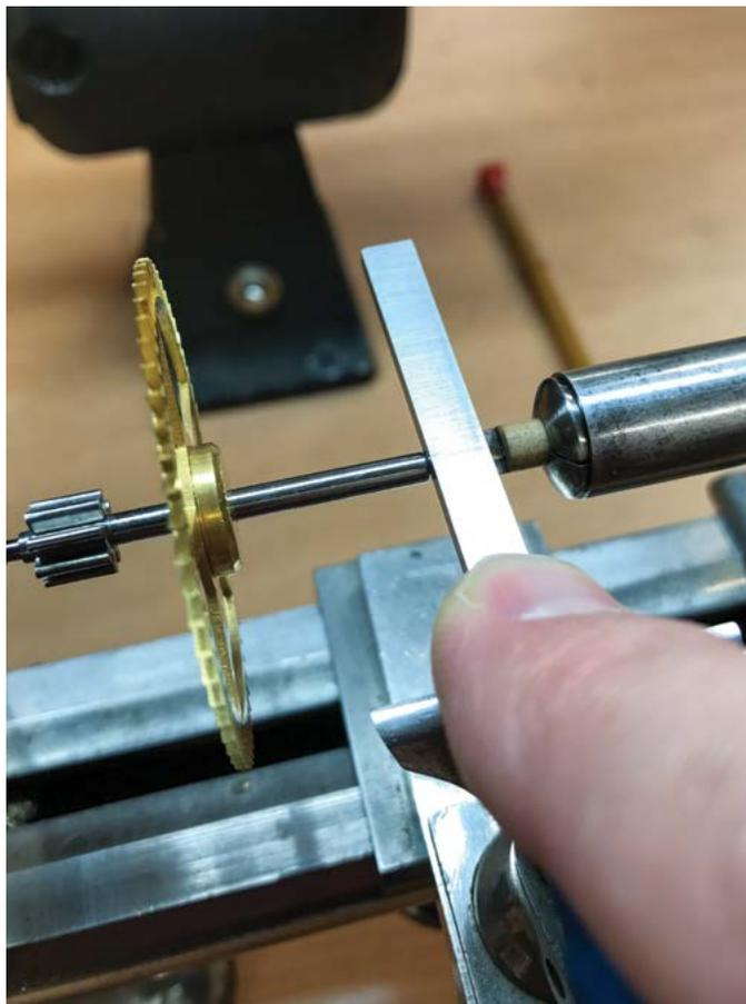
**Figure 1.** Setup for burnishing.
