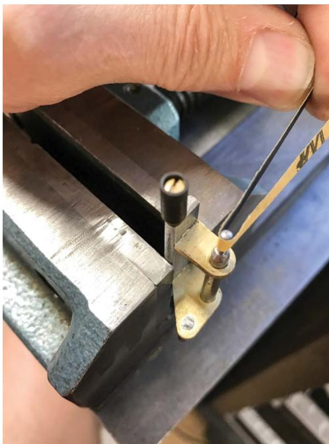
**Figure 9.** Removing wear and pre-polishing inaccessible pivots.
