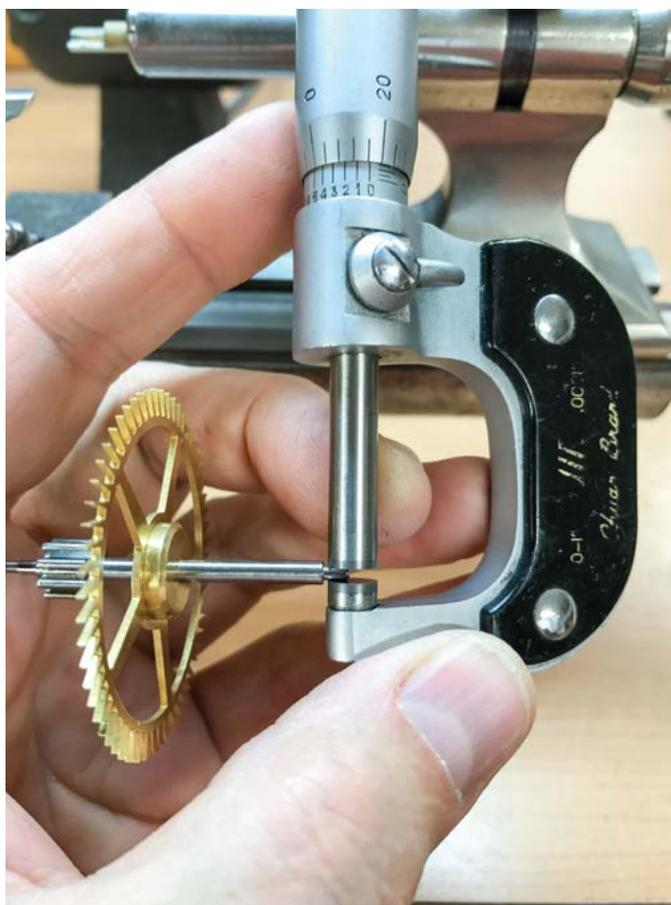
**Figure 5.** Checking for cylindrical pivot geometry near root; result is then compared to measurement near tip.
