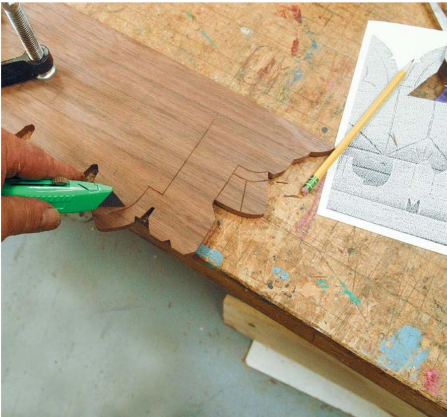
**Figure 5.** A C-clamp and utility knife are used in the carving process.
